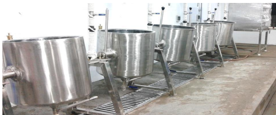
Idli Steamer (Gas / Electric) Cap. : 36 to 250 Itli
